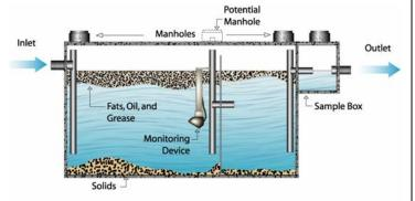
A grease interceptor should be checked and maintained to ensure that it is working properly. Backups, odors, and drainage problems are signs that the grease interceptor is not functioning as it should. See OC San's Fact Sheet for Grease Interceptor for specific tips on proper maintenance of grease interceptors.
