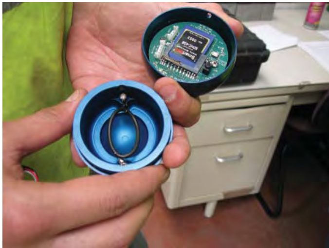
The SmartBall is a foam ball with an instrument in the center that records acoustic activity as it passes through a pipeline. The information gathered is analyzed to accurately pinpoint the size and location of any leaks or pockets of trapped gas in the pipe.
