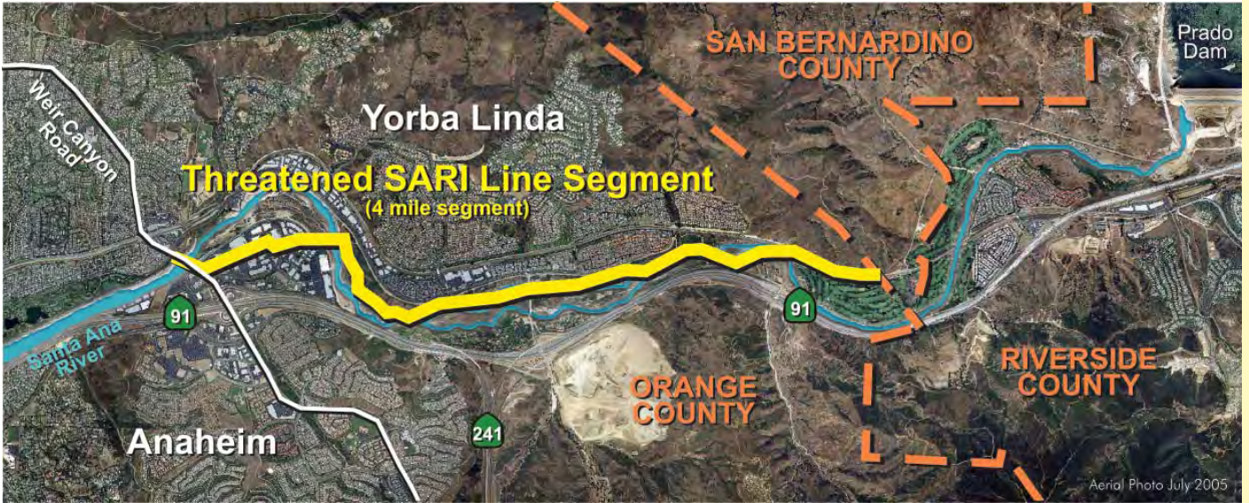
A four-mile segment of the Santa Ana River Interceptor pipeline will be rerouted out of the riverbed to protect the sewer system from erosion.
