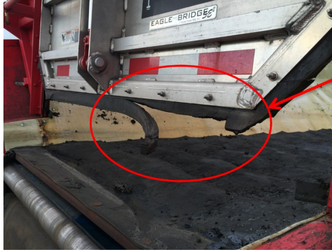
Unacceptable Damaged End Gate Seal
