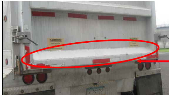
Missing Turnbuckles on bottom of gate.
